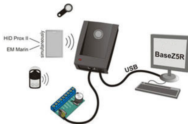
Figure 8. Wiring diagram for the Z-2 adapter (mod. E HTZ RF) to the controller and computer
